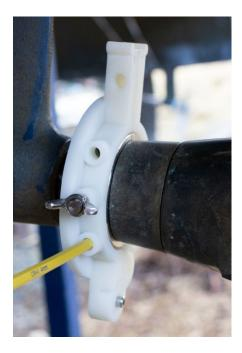
Check the alignment of the two halves as you tighten the bolts. There will be only a very small gap between the upper & lower section thanks to our precision design, which means the SeaSlicer<sup>™</sup> will be loose on your shaft until the final tightening.
