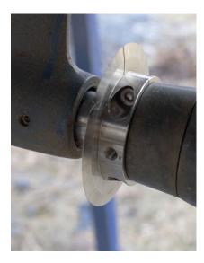
OPTIONAL: install the included set screws, which provide additional grip on your drive shaft. This may be required if your drive shaft is slightly undersized or was not fully clean.
